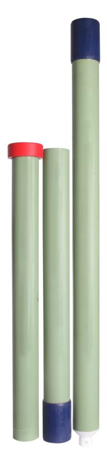
The ABS-60 QL inclinometer casing has four internal grooves and an integrated connection socket. It serves as a guide tube for driving an inclinometer probe or installing an inplace inclinometer. The connection socket of the ABS-60 QL (Quick Lock) makes it easy to quickly connect two tubes. Once the tubes are plugged together, all you have to do is insert a securing wire and the connection is complete.
