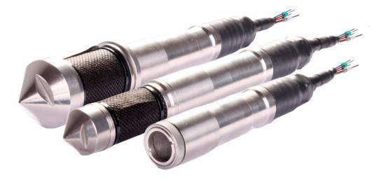
The transducers PW3 SV, PW3 RV and PW4 RV are sensors for water pressure measurement with a front or ring filter made of geotextile fleece. They are generally used to measure groundwater tables and also pore water pressure. Especially in soils with a high proportion of suspended particles or aggressive water, fleece filters are permanently permeable to water and ensure the monitoring operation.
