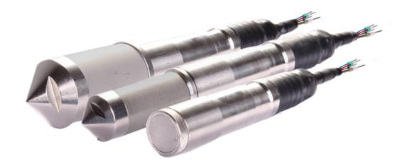
The sensors PP3 SS, PP3 RS and PP4 RS designate pore water pressure sensors with forehead or ring filters made of sintered metal. They are used to measure the groundwater level, the rock or pore water pressure in all disciplines of the construction industry. For demanding measurement tasks, piezometers with a ring filter are particularly suitable because of their large filter surface which ensures optimal contact with the water-saturated soil.
