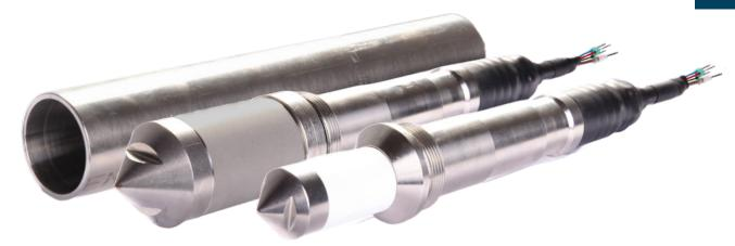
The sensors PP3 RK-E and PP4 RS-E designate pore water pressure transducers for pressing into soft soils suitable. For this type of installation, the sensors are particularly robust and have a connection thread to mount an press-in adapter. The outstanding feature is the ring filter made of ceramic or sintered metal with an extra large surface. The large filter surface ensures optimal contact with the water-saturated soil.
