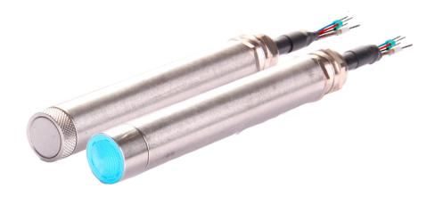
The pressure sensors PW 22 and PP 22 are used to measure water levels and pore water pressures. The slim design allows installation in boreholes or monitoring wells with a small diameter. For pure water level measurement in open standpipes the PW 22 with a plastic pre-filter is suitable. The PP 22 sensor is equipped with a sintered metal filter on the front and is used for pore water pressure measurements.
