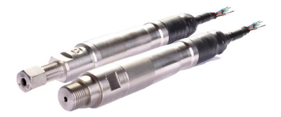
The PF-3 transducer series belongs to our pressure family and refers to sensors for measuring liquid pressures. These sensors can be connected to a fitting via the thread on the front and thus establish contact between the sensor membrane and the liquid pressure to be measured. The standard versions offer either a  $\frac{1}{2}$ " or an Ermeto 6S thread. Special adaptations and other threads are also available on request.
