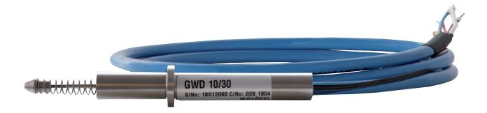
The displacement transducer GWD 10 is designed to provide maximum performance benefits within an extremely compact body diameter of 9.5 mm, with stroke lengths from 10 to 100mm. In most cases it is applied in fissuremeters and automatical measuring heads, type MA.
