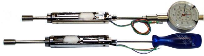
Figure: Displacement transducer type GWLO 22/60 with dial gauge and socket spanner
