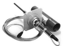
Fig: Head plate for extensioneter GKSE16 with assembled displacement transducer GWW (single extensioneter) with protection tube cover  $\varnothing$  90 mm, length = 46 cm
