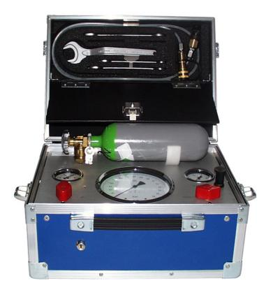
All components, inclusive a 200 bars/ 1 l compressed air cylinder are placed in a portable, splash-proof casing.
