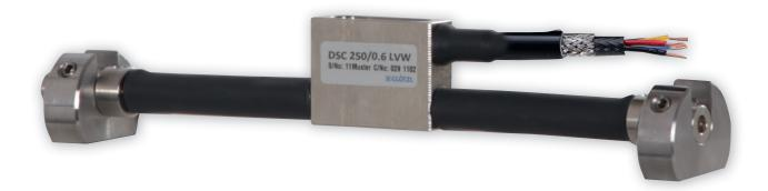
The vibrating wire strain gauge type DSC for arc welding to steel structures is commonly used for monitoring compression and/or tension in struts (excavation bracing), in structural members of buildings and bridges, girder constructions, sheet pile walls, tunnel linings and other steel structures.
