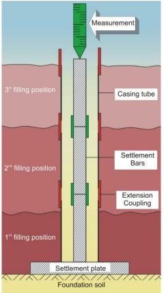
Plate settlement levels are simple auxiliary aids for the geodetic measurements to record the settlement in the backfill body and foundation base.
