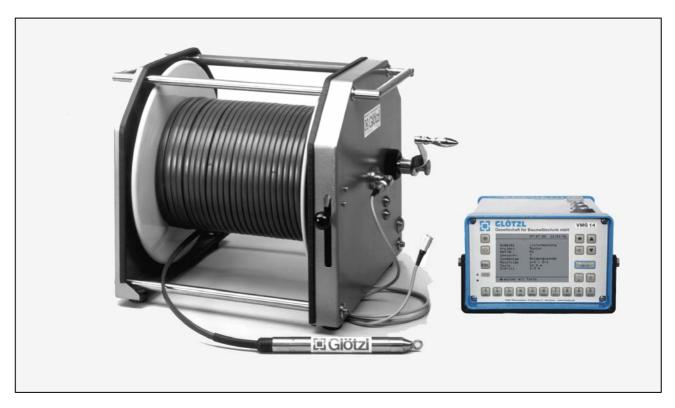
The hydrostatic profile gauge has been designed for measurement of the absolute height in horizontal resp. slightly horizontally inclined tubes. When passing the tubes with the measuring probe, the height difference between probe and a reference benchmark at tube beginning is determined at selected points. By comparison of two measuring series at different times, you get the settlement of the tube.
