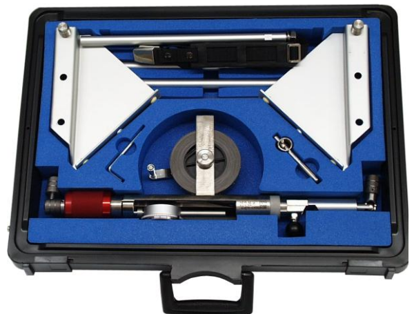
Figure: Convergence meas. device with meas. tape and dial gauge, test frame and assembly tool in transport case
