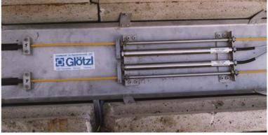
The displacement transducers of the series **GWD 20** are foreseen for installation in boreholes or also other application ranges where access is difficult. For this reason we did installation without electronic measuring amplifiers. When using the standard version, connection is made via Teflon wires which are grouted in the displacement transducer. Optionally, plug connectors are available. Evaluation electronics for processing of
