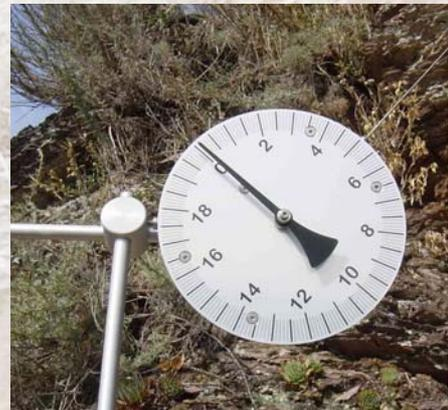
Assembly can very easily be done by means of dowels on the rock slope. The bars of the measuring device can be adapted and adjusted to the spacious conditions in all possible directions.
