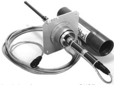
Fig: Head plate for extensometer GKSE16 with assembled displacement transducer GWW (single extensometer) with protection tube cover  $\varnothing$  90 mm, length = 46 cm
