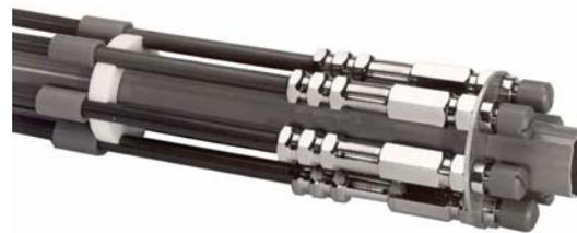
Figure: 6-fold extensometer head, type GKSE 6/16, consisting of inclination measuring tube with 6 single extensometers, foldaway assembly plate for installation in boreholes. For fixing the extensometers around the inclination measuring tubes, corresponding plastic holders are available.
