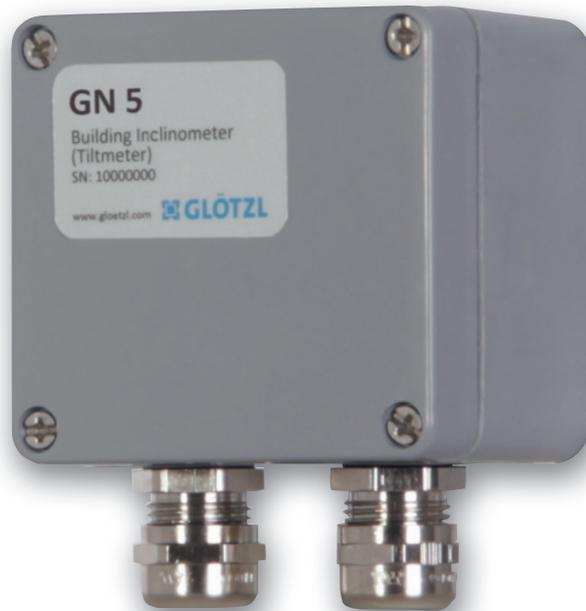
The GN 5 compact building inclinometer features precise inclinometer sensors with a restricted measuring range of  $\pm 5^\circ$  and a resolution of 0.02 mm/m for measured values. It is used to record inclination changes in buildings. Equipped with a sensor for measuring axis x and a temperature sensor, the GN 5/1 tiltmeter device records inclinations at right angles to the mounting surface, while the GN 5/2 2-axis sensor measures in both x and y directions.
