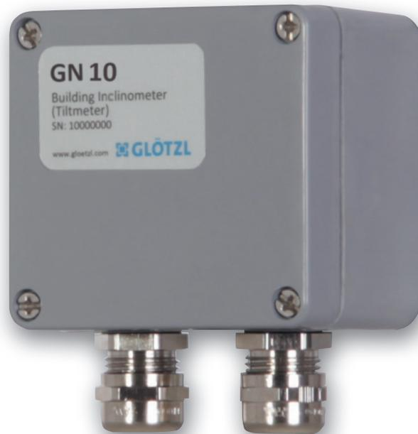
The GN 10 compact building inclinometer features precise inclinometer sensors with a restricted measuring range of  $\pm 10^\circ$  and a resolution of 0.02 mm/m for measured values. It is used to record inclination changes in buildings. Equipped with a sensor for measuring axis x and a temperature sensor, the GN 10/1 tiltmeter records inclinations at right angles to the mounting surface, while the GN 10/2 2-axis sensor measures in both x and y directions.
