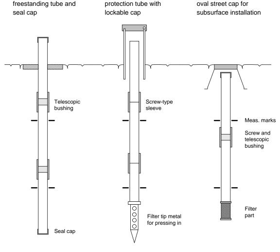
Inclination measuring tube PVC in connection with measuring marks, telescopic bushings for intake of settlements Further details see inclination measuring tube.
