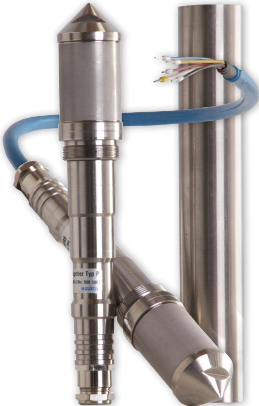
This kind of piezometer Type PP4 RS is the heavy-duty model with an extra-large ring filter made of sintered metal. The model PP4 RS E is a push-in Piezometer which can be pushed directly into soft soils.
